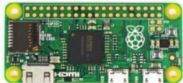
Figura 6. Placa Raspberry Pi Zero
